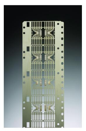
LOC The Lead On Chip features lead fingers that are attached directly to the surface of the chip using a double-sided adhesive tape. Since there is no die pad on the LOC lead frame, the package allows for higher density, enabling it to accommodate a larger IC chip and providing better reliability performance than traditional packages.
