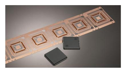
PLCC The Plastic Leaded Chip Carrier has leads on all four sides with J-shaped bends and is available with a variety of pad designs, such as dual-pad. Designs with fused leads promote better thermal performance, while those with a closed dambar reduce mold flash and improve the solder plating coverage.
