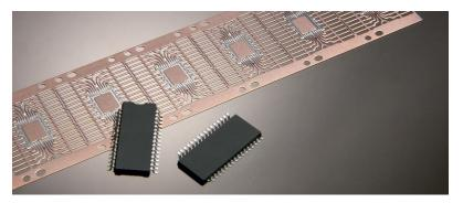
SOIC The Small Outline Integrated Circuit is available in a number of variations, including SOP (Small Outline Package), SSOP (Shrink Small Outline Package), SOJ (Small Outline J-Leaded), TSOP (Thin Small Outline Package), and TSSOP (Thin Shrink Small Outline Package). The SOIC package is desirable for its small footprint on the circuit board. SO lead frames are available in single-pad, dual-pad and matrix designs.
