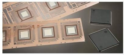
QFP/TQFP The Quad Flat Pack/Thin Quad Flat Pack is a plastic package with a square or rectangular body with leads on all four sides in a gull-wing configuration. Designs with "dimples" (half-etched holes) on the back side of the pad provide the mechanical adhesion to prevent delamination. Different pad designs exist to further enhance package reliability, while designs with a dual-pad lead frame are available to minimize cost.
